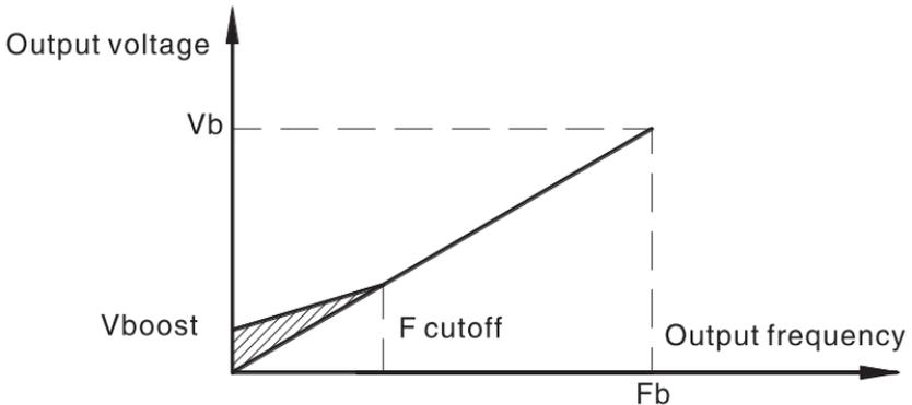
Figure 6-9(1) Manual torque boost diagram
