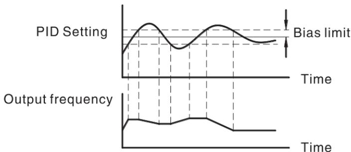
Figure 6-23 Bias limit action diagram
