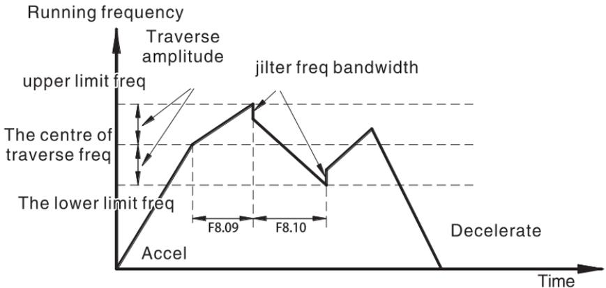
Figure6-18 Traverse operation diagram
