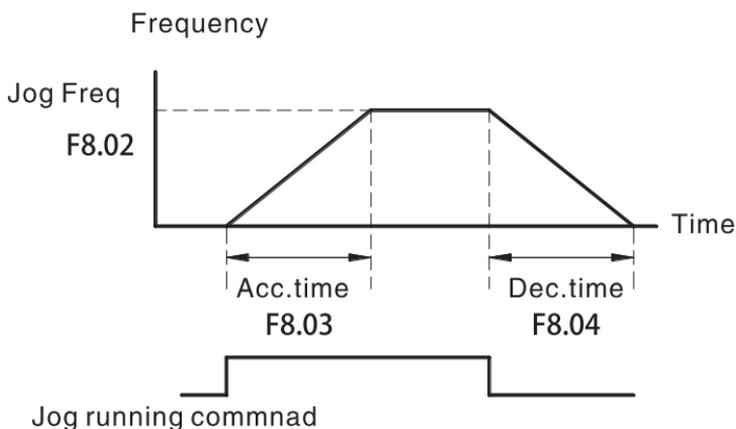
Figure 6-16 Jog running frequency and Acc./Dec. time
