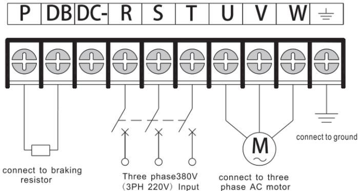
Fig.3-21 Diagram 4 for Main Circuit Terminals
