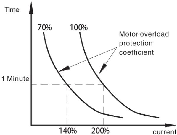
Figure 6-28 Motor overload protection curve
