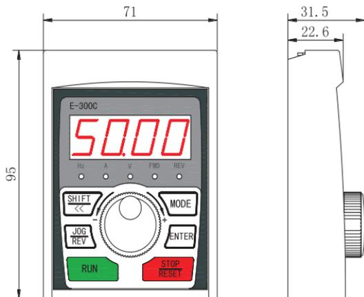
Fig. 9 – 4 Dimension of E-300 keypad
