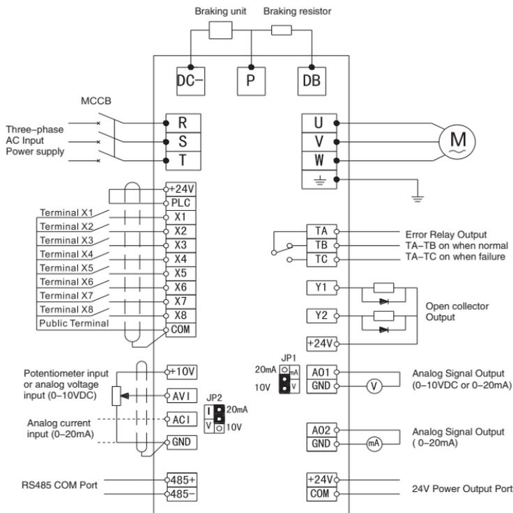
Fig.3-16 Basic wiring diagram
