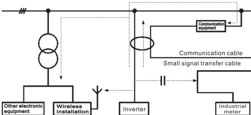
Propagation Diagram of Input Cable's Interference over External Equipment
