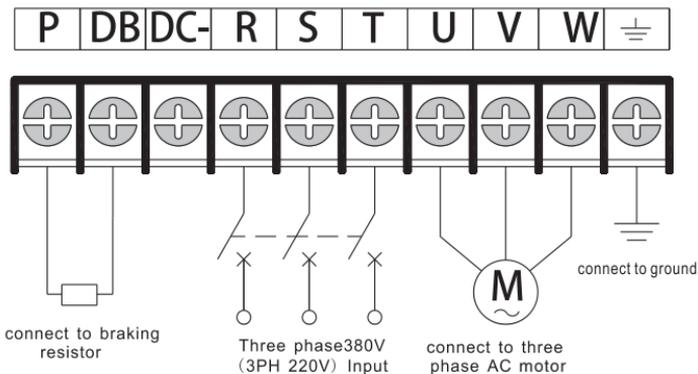
Fig.3-21 Diagram 4 for Main Circuit Terminals
