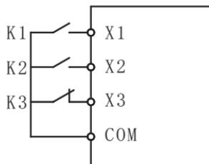
Fig.6-12 3-wire control mode diagram
