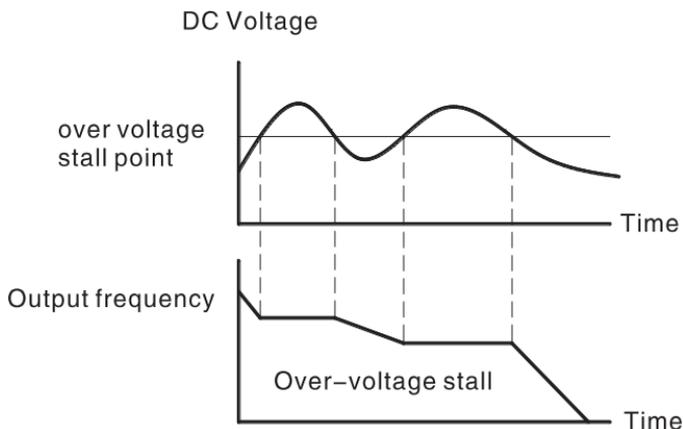
Figure 6-29 Over voltage stall function
