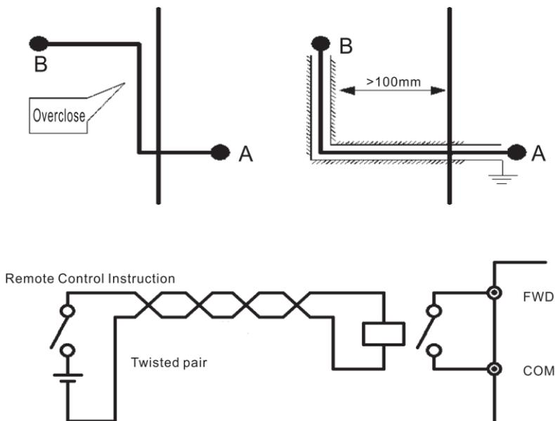
3. This type of interference can be suppressed by a good earth ground of the
