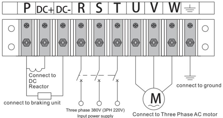
Fig.3-23 Diagram 6 for Main Circuit Terminals
