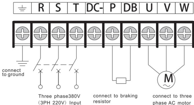
Fig.3-20 Diagram 3 for Main Circuit Terminals
