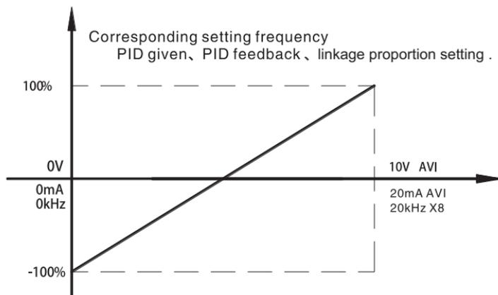
Figure 6-13 Analog given and setting
