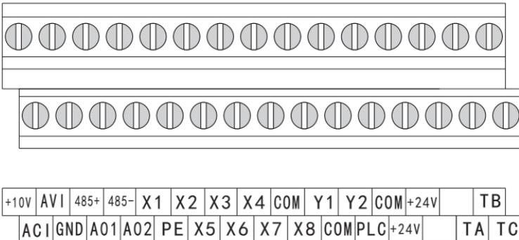
Fig.3-25 Control Circuit Terminals (2)
