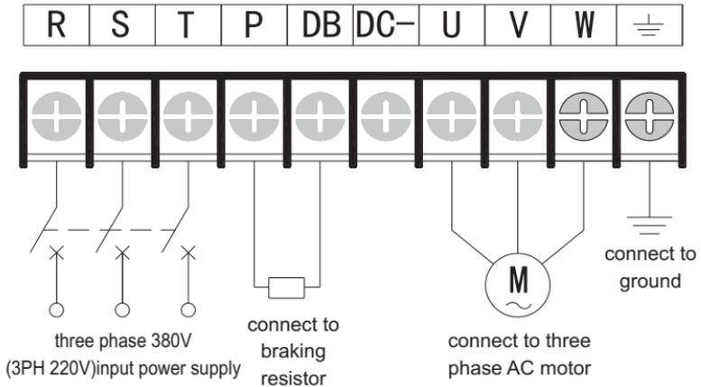
Fig.3-22 Diagram 5 for Main Circuit Terminals
