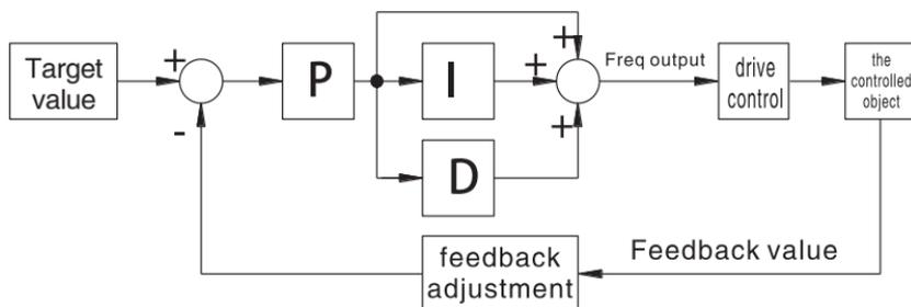
Figure 6-22 PID control diagram
