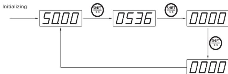
② Modification of function parameter value (Modify the parameter value of F8.02 JOG frequency value from 5.00hz to 20.00 Hz)
