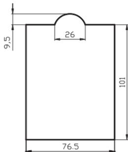
Fig.9 – 5 Hole dimension 1 of keypad.
