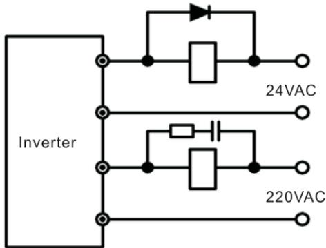
As for a 24VDC controlled relay a shunt winding continuous current diode should be inserted at both ends of the coil and pay attention to the polarity of diode. As for a 220V AC controlled contactor; an over-voltage suppressor should be mounted at both ends of the coil (i.e., RC network). Also, the protection of switch contact can not be ignored. This can be realized by forming a shunt winding RC or RCD buffered network, as shown in the figure below
