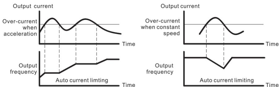
Fig 6-30 Auto current limiting function
