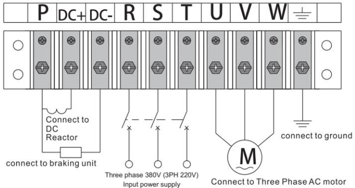
Fig.3-23 Diagram 6 for Main Circuit Terminals
