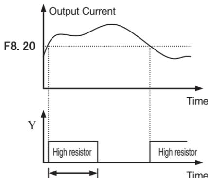
Fig.6-21 Overload pre-alarm schematic
