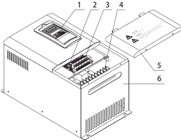
**Figure 2-6 Model B Structural Representation**
