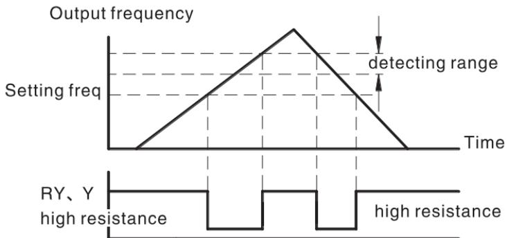
Figure 6-20 Frequency arriving detecting diagram
