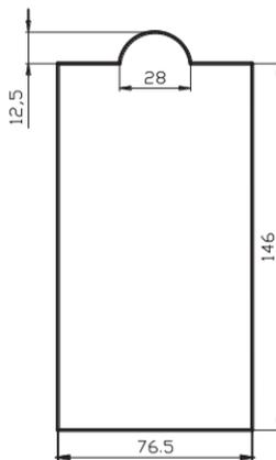
Fig.9 – 6 Hole dimension 2 of keypad
