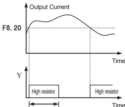
Fig.6-21 Overload pre-alarm schematic
