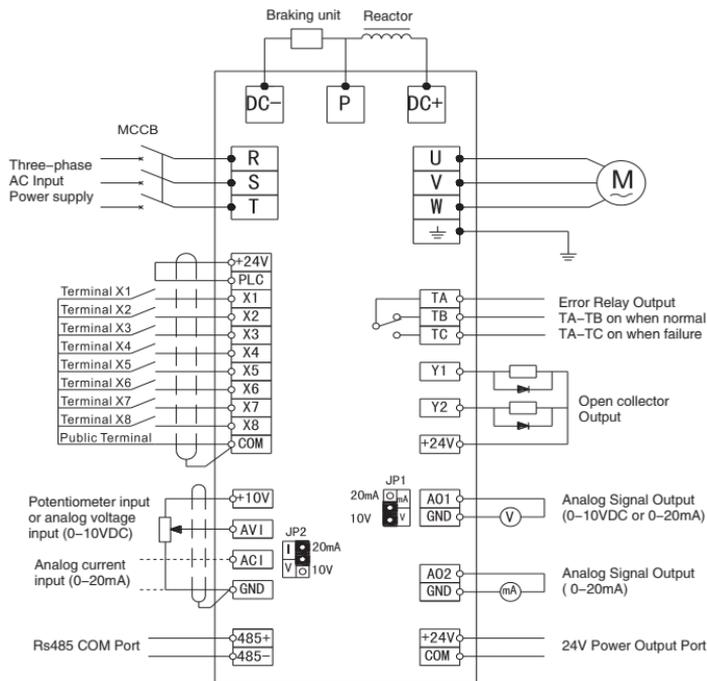
Fig. 3-17 Basic wiring diagram
