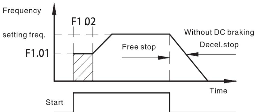
Figure 6-4 Start and stop frequency output curve
