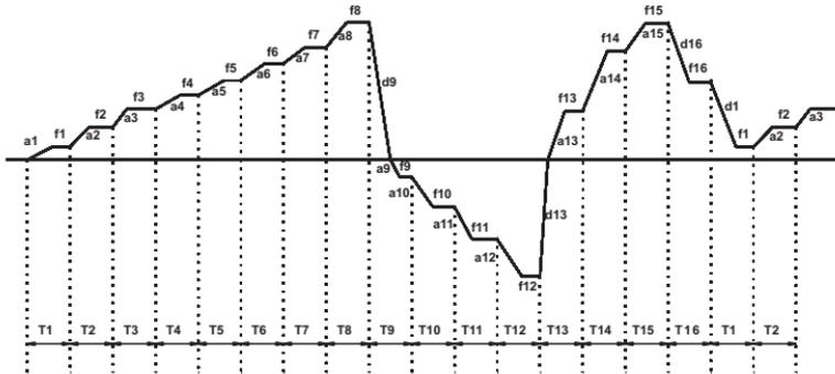
Fig.6-26 PLC / multi-speed continuous cycle running
